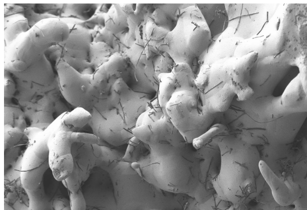
Fig.24. Silver base composite reinforced by carbon nanotubes. (Courtesy of ITME)
