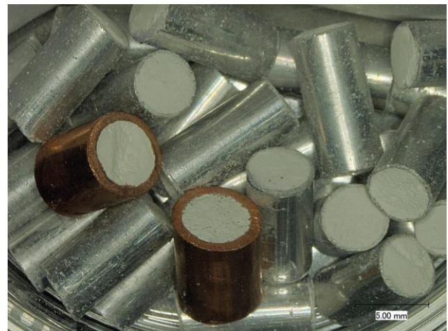
Fig.9. Al and copper-coated zeolite pellets to improve thermal conductivity in heat storage applications. (Courtesy of IKTS)
