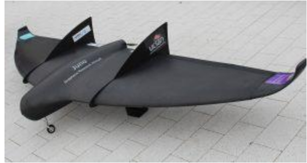
Fig.20. Juno world’s first graphene skinned plane. (Courtesy of Haydale)
