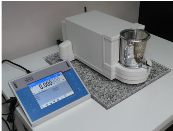
Fig. 19. High resolution ( 1\mu\text{g} ) microbalance (courtesy of AGH-UST).
