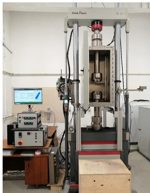
Fig. 12. Complex for determination of mechanical characteristics and crack resistance in static and dynamic conditions in wide temperature range (courtesy of IMBAS).
