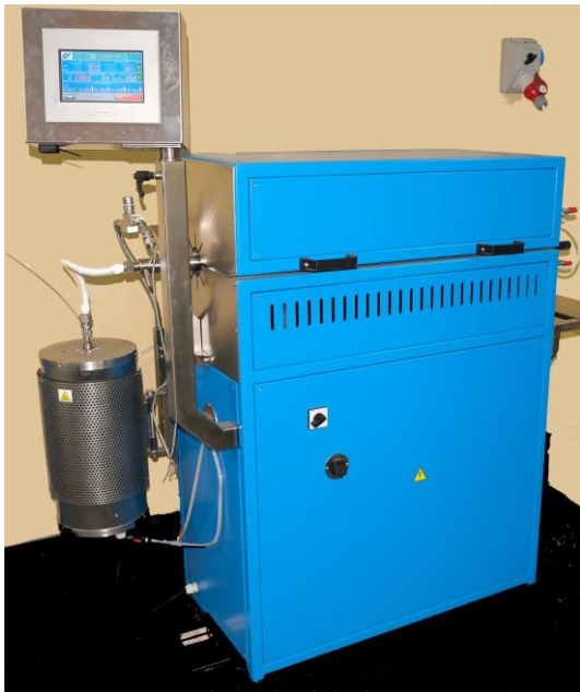
Fig. 18. Digitally controlled, advanced oxidation test stand (courtesy of AGH-UST).
